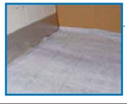
The floor cover material should extend to the side walls. The floor cover along with the foam blocks prevent freezing air from circulating under the bulkhead into the chilled section. You are now ready to load your Chilled Cargo. Laminated floor material is tough enough to load pallets with a forklift without tearing.
