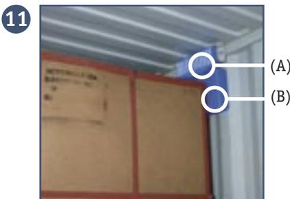
The upper part of the housing (A) contains the salt and must be exposed to the air. The lower part (B) can be covered with cargo if necessary.
