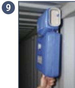
hold the bottom part of the hook rod and push the blue housing all the way up to the ceiling.
