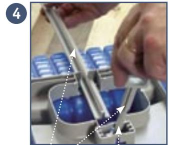
Insert the hook bar (A) halfway into the bracket (D) from the top...and lower the threaded rod (B) through the bracket (D) into the hole in the ABSORTOP® leaving only the top of the threaded rod (B) exposed.
